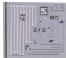
Efficient sample introduction. Silicon micro-machined, variable volume injector introduces sample in a narrow band.
