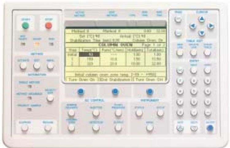
Navigate method parameters. Use section-specific soft keys to access and edit method parameters independent of PC workstation.
